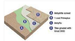
Anhydrite screed must be confirmed dry via consistent moisture readings before tiling commences. The residual moisture content must be less than 0.5% or 75% relative humidity (RH).
