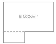
Joint required as the corner makes up over 50% of the area's length.
