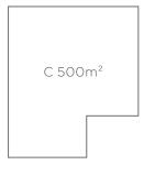
No joint required unless specified as a construction or day joint. Corner is under 50% of length.
